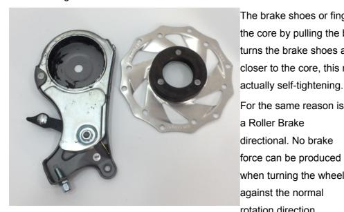
The brake shoes or fingers are tighten around the core by pulling the brake lever. As the core turns the brake shoes are getting dragged closer to the core, this means the brake is
